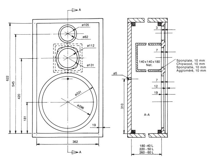
Alle mål i mm. All measures in mm. Alle Masse in mm. Toutes mesures en mm. Sponplate, 19 mm Chipwood, 19 mm Sponplatte, 19 mm Aggloméré, 19 mm
