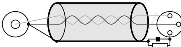
The RC network (100nF, 100 ohms) can usually be shorted since consumer kit is always ground lifted. After all, it's the only thing that will have at least *some* effect when you only have 1 wire for the signal and the reference is sort of democratically negotiated among the boxes in the rig. This of course is why some pro designers were primed to think along those lines instead of just letting go of the whole "audio ground think" entirely.
