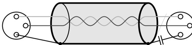
This serves to illustrate once again that the pin 1 problem is entirely self-inflicted. *There simply is no reason why, in a balanced connection, the two "audio grounds" should be connected by the audio cable.* So long as the two circuits are within volts from each other the whole set-up will work wonderfully.
