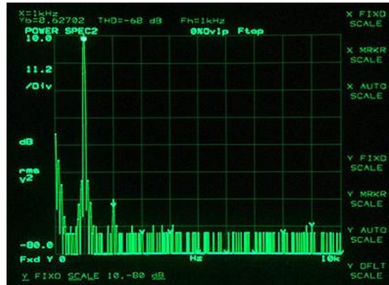
This trace shows the output harmonic spectrum of 10KHz at 1W into 8 ohm load. GlowMaster shows amazing low distortion -68dB (0.039%) same level for 1KHz. This is not easy for other amplifiers to achieve where 1KHz performance may be good, but start to get high distortion at higher frequency.
