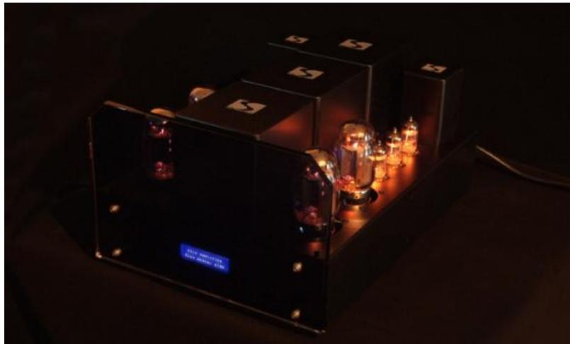
New GlowMaster KT-88 features high quality parts through out the circuit. Point to point hand wiring is used for all signal path to maximise the signal transmission. SAC uses high quality Amphenol XLR input, Gold plated RCA, Heavy duty gold plated (insulated) binding post, Miyama switch, OFC bus wire, silver solder and best of all, the new SILK P-4200 Balanced output transformer. Power transformer is SILK handwound with special electro-static shield and electro-magnetic shield.
