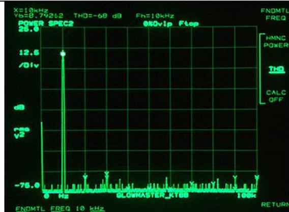
This trace shows harmonic spectrum of a 1KHz signal at 65w into an 8 ohm load. Amazing low distortion of -56dB is obtained
