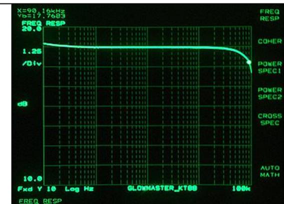
The Frequency response at 65 watt is linear within 0.1dB from 20Hz to 20,000Hz. This is better than most solid state amplifiers (which already use high amounts of negative feedback). The level of accuracy of new GlowMaster KT-88 is only available in reference instruments, which set a new class of its own.
