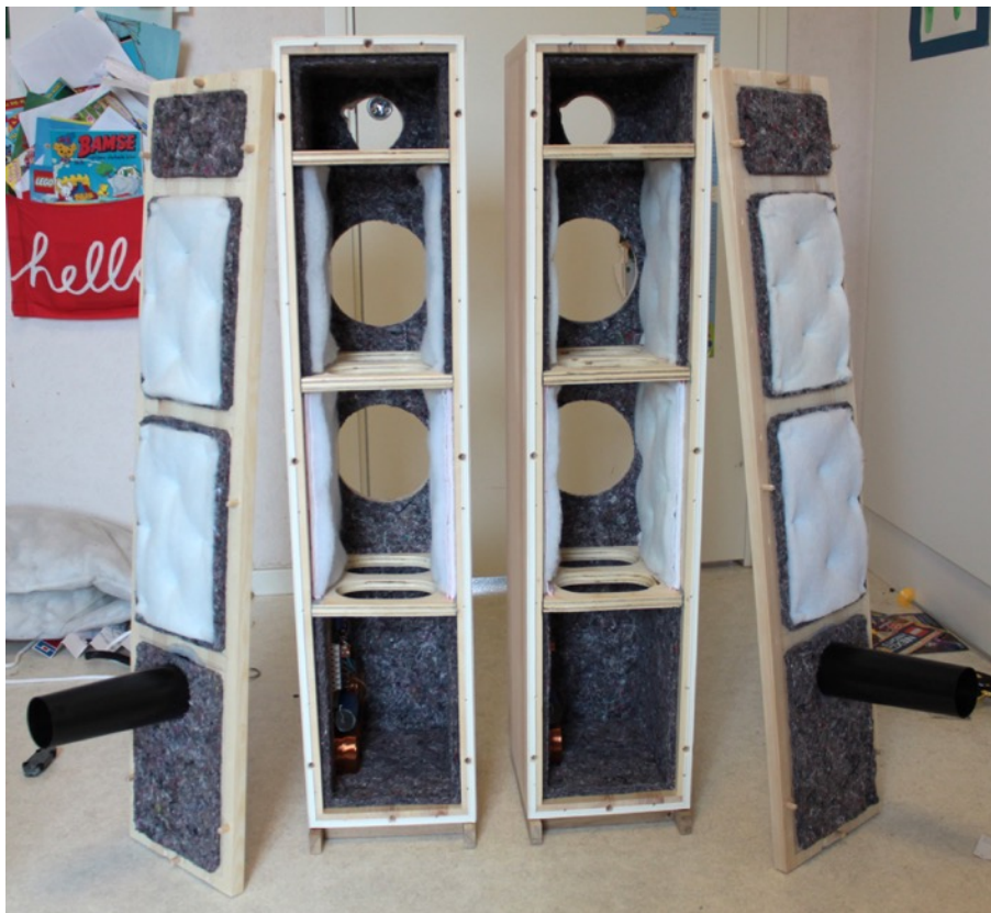
Damping installed (ports not cut to correct length)
