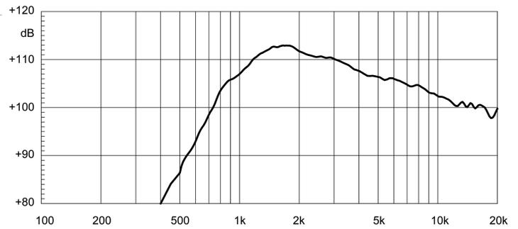
NSD1095N MEASURED WITH 1W INPUT ON RATED IMPEDANCE AT 1M DISTANCE ON XT1086 HORN MOUTH AXIS
