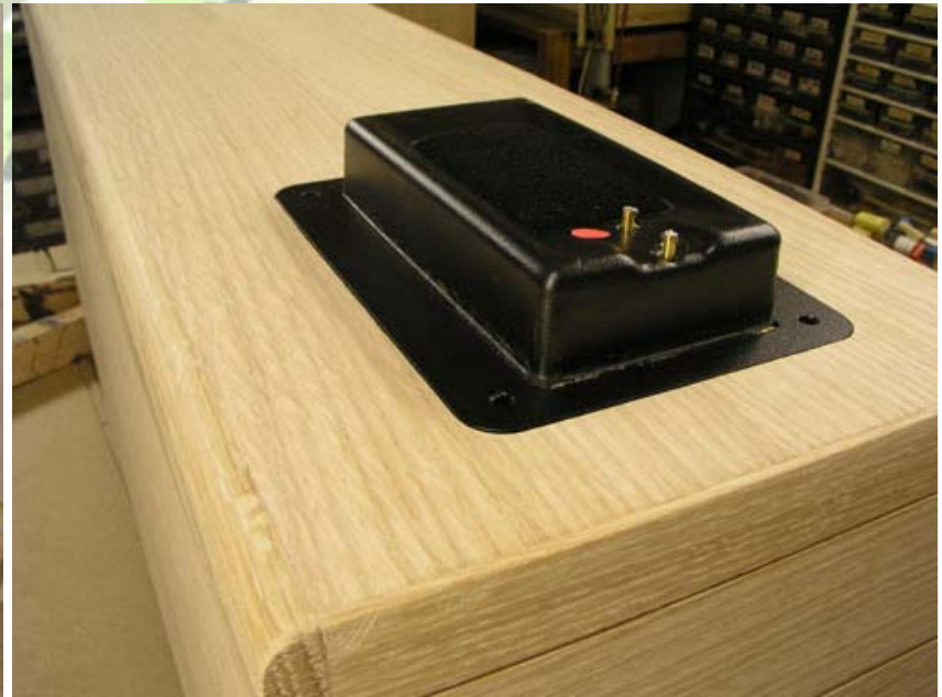
Routing for the Raidho tweeter. Use a 19-20 mm router bit to fit tweeter corners.
