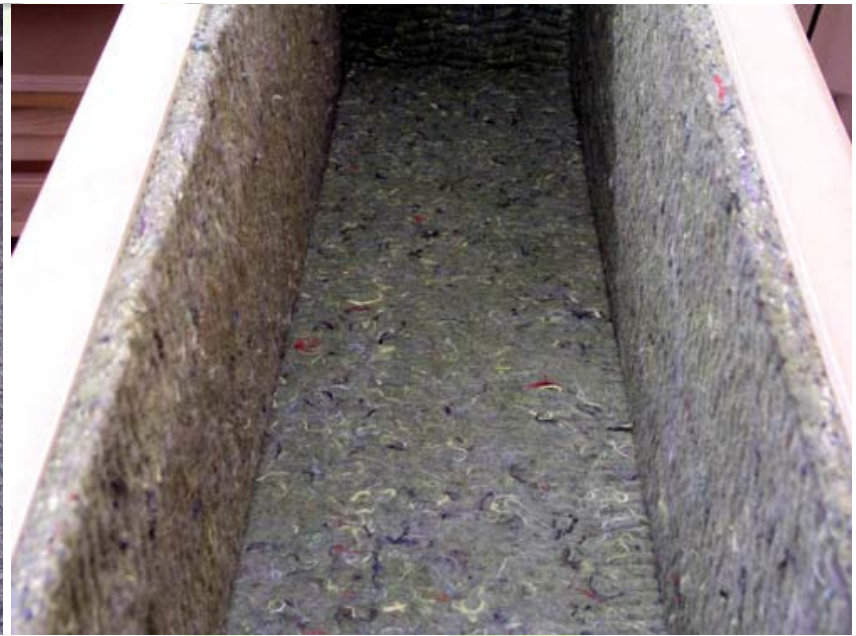
10 mm felt material used for basic damping of interior.
