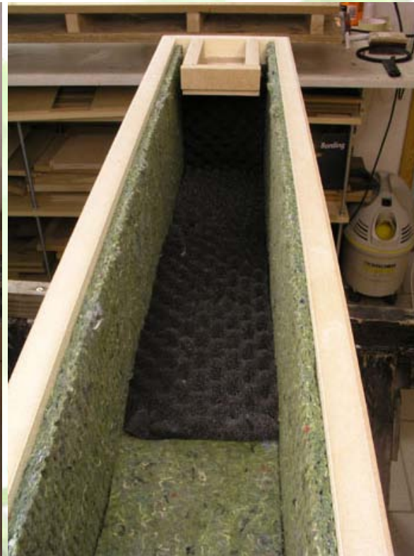
Use 20 mm egg crate foam or MDM3 as additional damping behind drivers.
