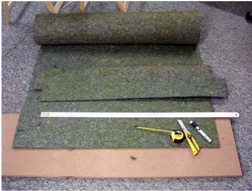
10 mm felt material used for basic damping of interior.
