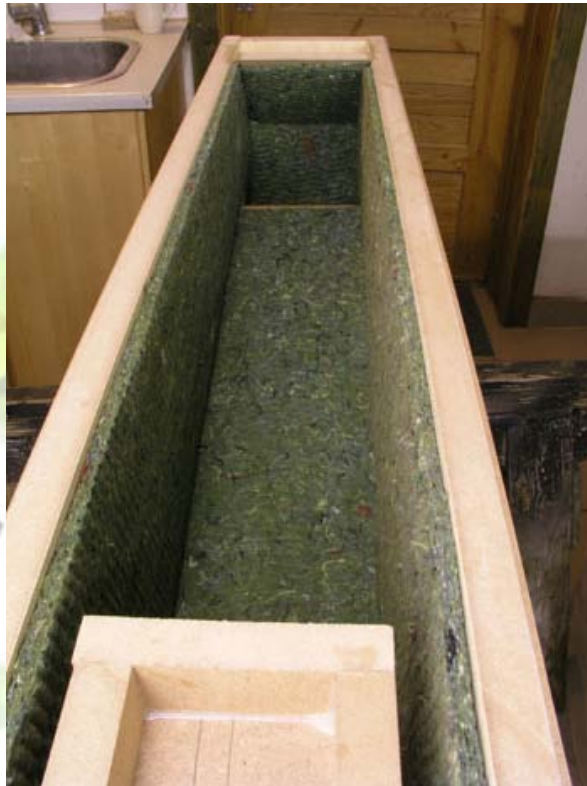
Use 20 mm egg crate foam or MDM3 as additional damping behind drivers.
