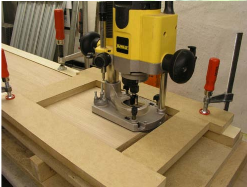
Routing for the Raidho tweeter. Use a 19-20 mm router bit to fit tweeter corners.
