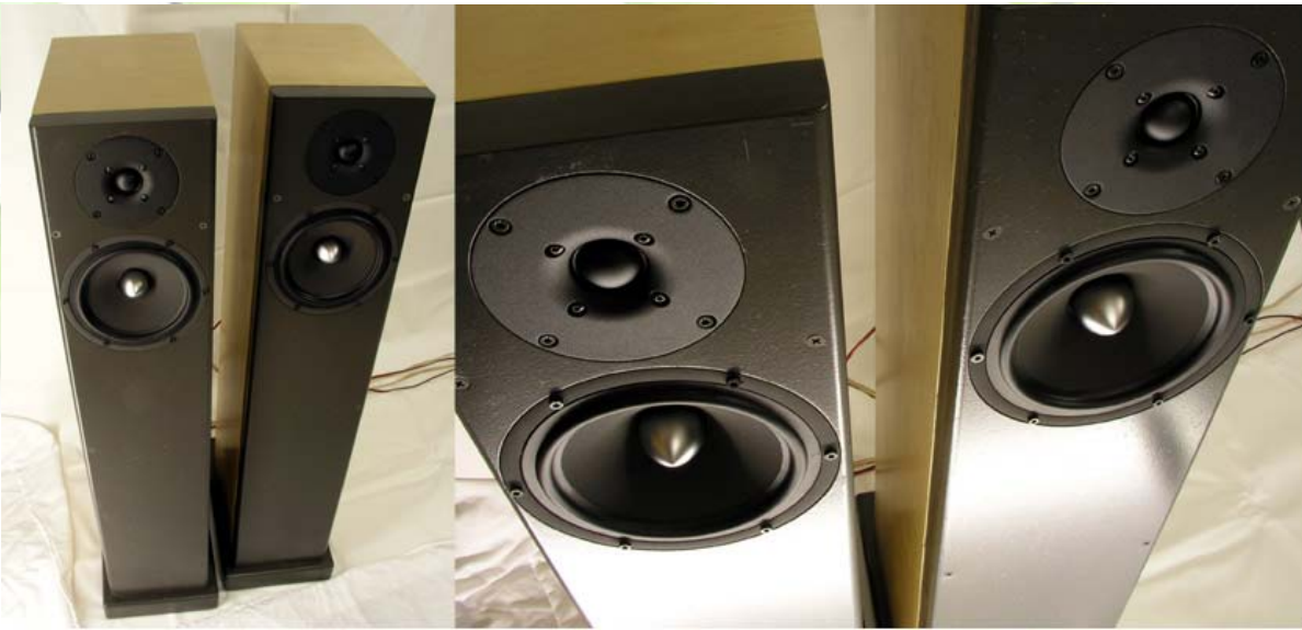
CNO-T25 testcabs. 2 x 16 mm MDF laminated for front panels. Remember to chamfer W18 driver hole well for proper rear ventilation!
